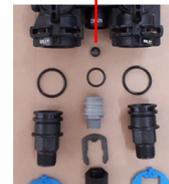
During the assembling valve, always verify the presence of the rubber ball, which is essential for a correct drainage of the water flow during washing cycles.
